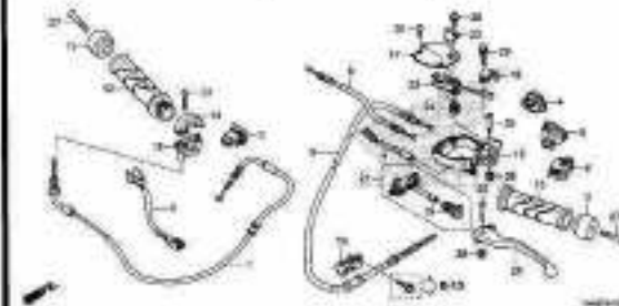
F-4-10 HANDLE LEVER/SWITCH/CABLE (ACI110CBE)
